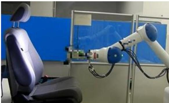
Appearance quality is currently judged by humans. AI visual inspection can realize labor saving and quality stabilization by unmanned inspection.
